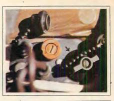
Close-up of power-pack on typical infrared device. Is mounted in backpack assembly with 6-volt power source. Knob at lower right (see arrow) is off-on switch. Output cables to both IR light source and electronic telescope are located at lower left. Manipulation of switch is made easy by location in opening in bottom of backpack.
